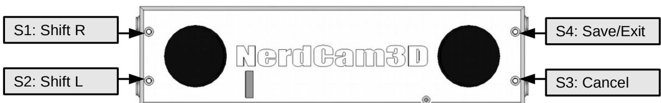
Figure 10: Push button functions for squeezed side-by-side offset adjustment
