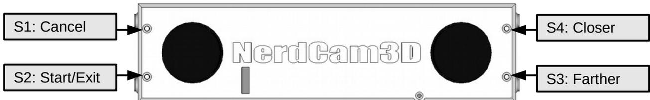
Figure 6: Push button functions for 3D-OSD convergence adjustment
