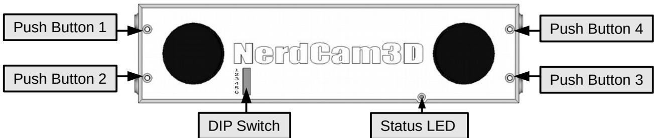
**Figure 1: Control elements on front side**
