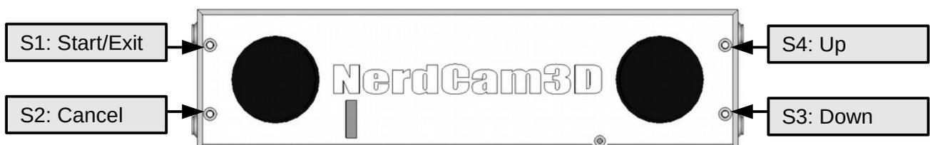
Figure 5: Push button functions for vertical sensor adjustment
