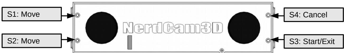
Figure 8: Push button functions for cropped side-by-side offset adjustment
