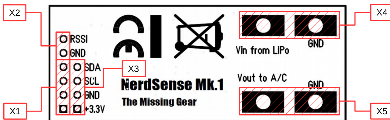
Figure 5: Overview of sensor interfaces
