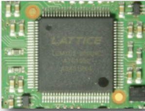
Advanced video processing with FPGA for minimum signal latency. No additional video frame buffer required.
